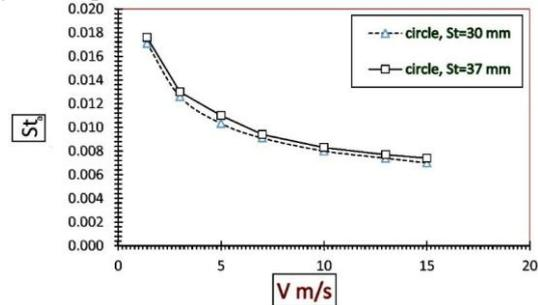
Fig. 12. Effect of longitudinal pitch on  $St_a$  for circular cross section.
