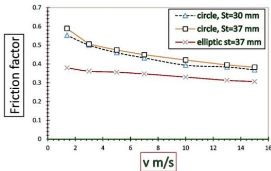
Fig. 18. Effect of tube cross section on friction coefficient.
