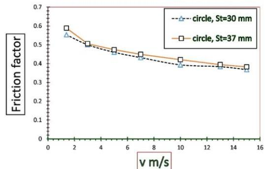
Fig. 14. Effect of longitudinal pitch on friction coefficient for circular cross section.
