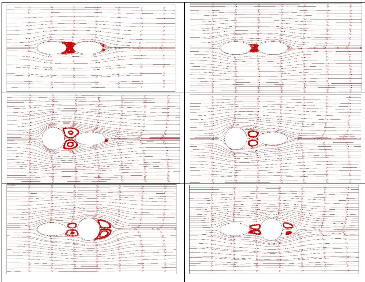
Fig. 6. Streamlines patterns of the tested tubes at different arrangements.
