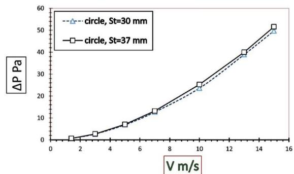
Fig. 13. Effect of longitudinal pitch on  $\Delta P$  (Pa) for circular cross section.
