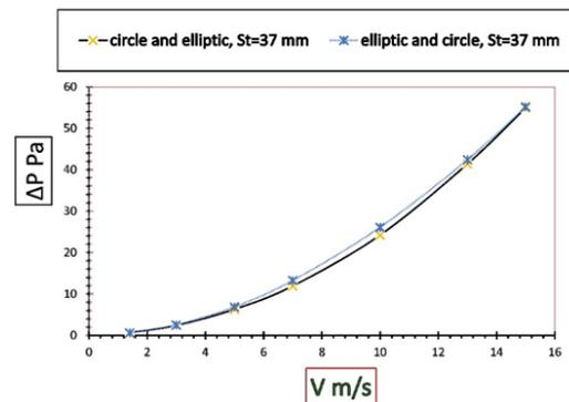
Fig. 21. Effect of tube arrangement on  $\Delta P$  (Pa).
