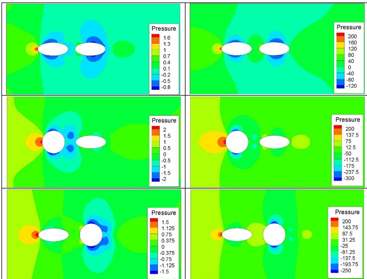
**Fig. 10.** Static pressure (Pa) contours at different arrangements.
