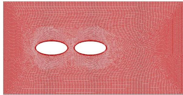
**Fig. 4.** Mesh Configurations for the Domain of the Tubes.
