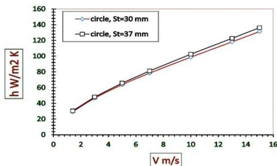
Fig. 11. Effect of longitudinal pitch on  $h$  (W/m<sup>2</sup>K) for circular cross section.
