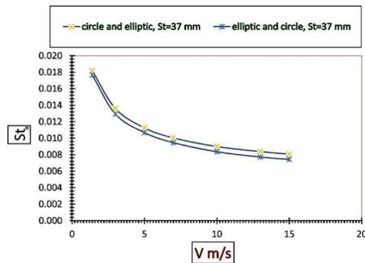
Fig. 20. Effect of tube arrangement on  $St_a$ .
