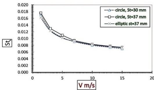
Fig. 16. Effect of tube cross section on  $St_a$ .
