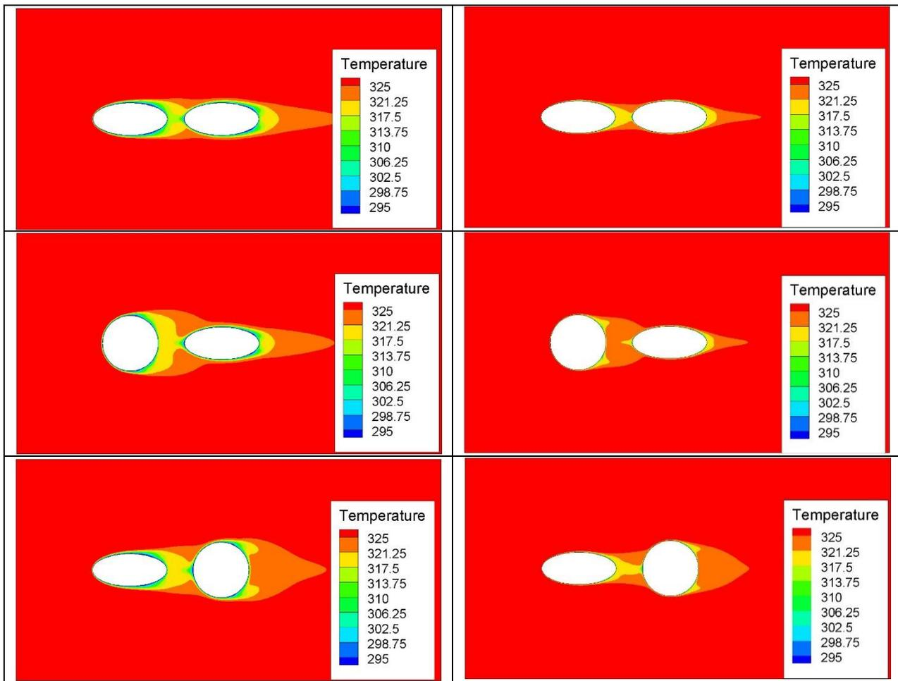
Fig. 9. Temperature (K) contours for different arrangements.
