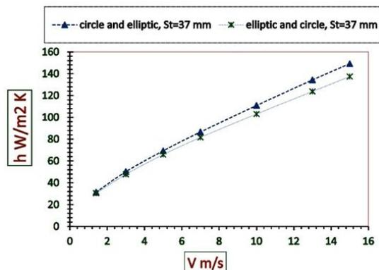
Fig. 19. Effect of tube arrangement on  $h$  (W/m<sup>2</sup>K).
