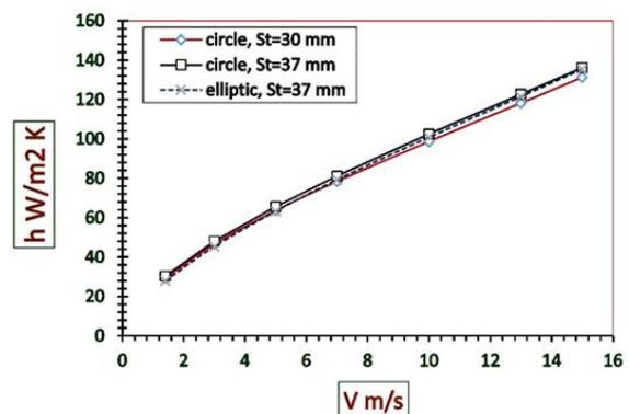
Fig. 15. Effect of tube cross section on  $h$  (W/m<sup>2</sup>K).
