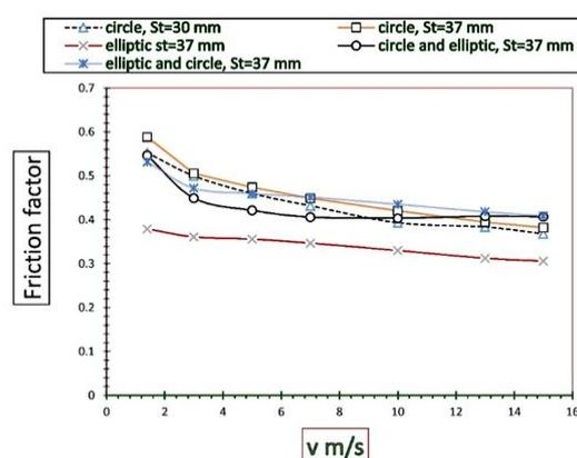
Fig. 26. Friction coefficient vs.  $V$  (m/s) for different studied arrangement.
