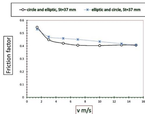
Fig. 22. Effect of tube arrangement on friction coefficient.
