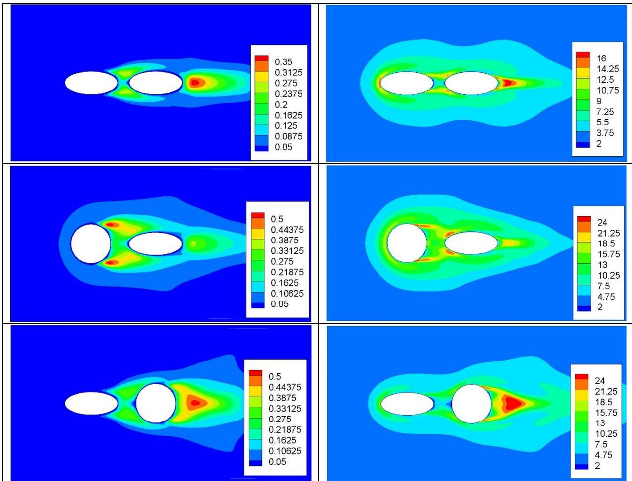
Fig. 8. Turbulent kinetic energy contours for different arrangements.
