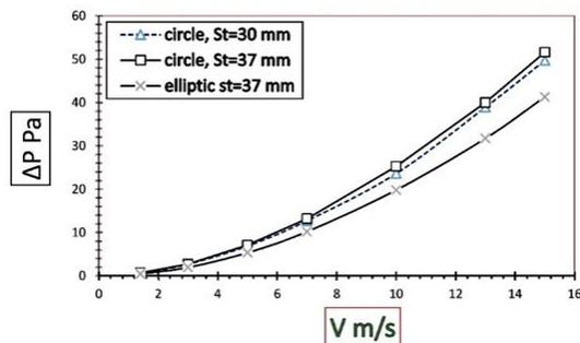
Fig. 17. Effect of tube cross section on  $\Delta P$  (Pa).
