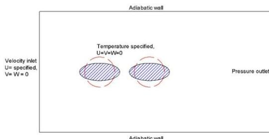
**Fig.3.** Boundary conditions for the numerical domain.
